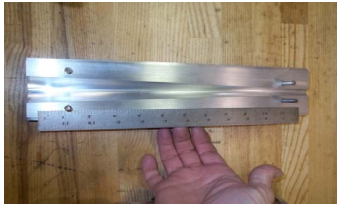
Figure 3.6 Diffuser designed for the upflow column
