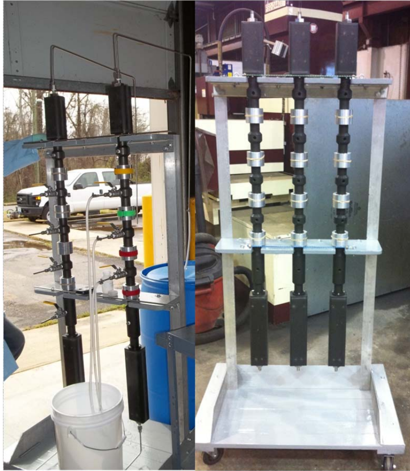
Figure 3.8 Upflow column setup
