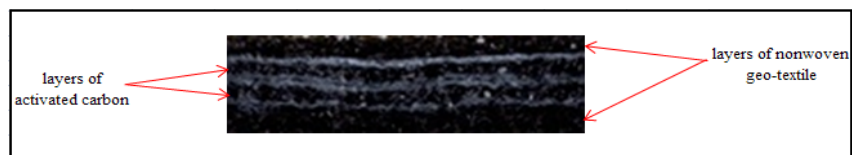
Figure 3.2 FilterMat™ with two layers of nonwoven geotextile and activated carbon
